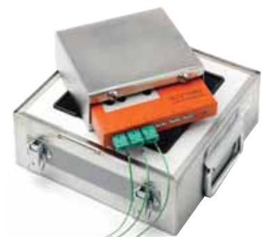
Incorrect: Probe leads are twisted
