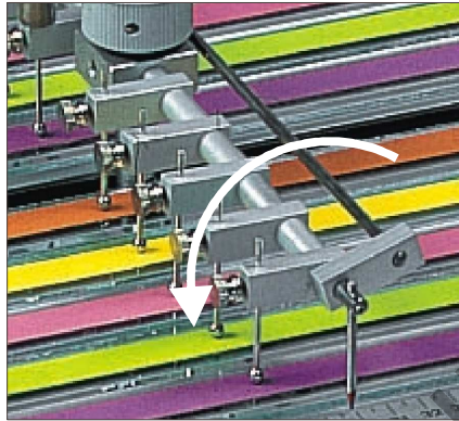
Figure 3. Rotate the balls down onto the specimens
