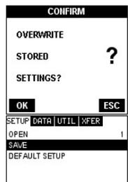
setup file in your gauge was somehow corrupted, and you do not have immediate access to a computer to re-load the factory setup back into the gauge. This gives you the ability to load and modify a basic setup as follows:
