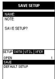
*Note: The Name and Note parameters of a Setup can be edited at any time by repeating the Save Setup routine described above. Therefore, the Save Setup function can also be considered an Edit Function.*
